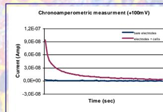
Fig. 4. Chronoamperometric response of N2a cells at +100mV in PBS (60µl). Bare PEDOT/Nafion/Polylysine electrodes showed no difference in current response, while cells produced sharp decreases from their initial currents.
