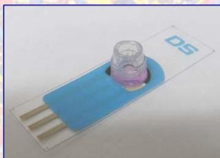
Fig. 2. Cell culture well on top of PEDOT electrode consisting of a cut-off pipette tip (polystyrene, diameter 4mm)
